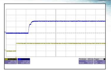
Figure 8: Turn-on transient at full resistive load and zero output capacitance initiated by Vin. ON/OFF Pin previously low. Ch 1: Vout (5V/div). Ch 3: Vin (200V/div).
