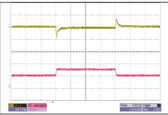
**Figure 11:** Output voltage response to step-change in load current (50%-75%-50% of lout(max);  $dI/dt = 0.1 A/\mu s$ ). Load cap: 1  $\mu$ F ceramic and 15  $\mu$ F tantalum capacitors. Ch 1: Vout (200mV/div), Ch 2: lout (20A/div).
