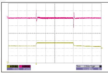
**Figure 12:** Output voltage response to step-change in input voltage (250V/ms). Load cap: 100  $\mu$ F electrolytic output capacitance. Ch 1: Vin (100V/div), Ch 2: Vout (200mV/div).
