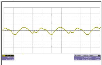
**Figure 10:** Output voltage ripple, Vout, at nominal input voltage and rated load current (200 mV/div). Load capacitance:  $1\mu F$  ceramic capacitor and  $10\mu F$  tantalum capacitor. Bandwidth: 10 MHz. See Figure 17.
