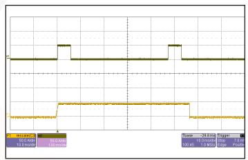
Figure 18: Load current (50A/div) as a function of time (10ms/div and 100ms/ div) when the converter attempts to turn on into a 10 m $\Omega$  short circuit.
