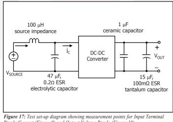
Ripple Current (Figure 9) and Output Voltage Ripple (Figure 10).
