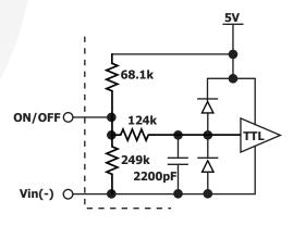
Figure B: Internal ON/OFF pin circuitry
